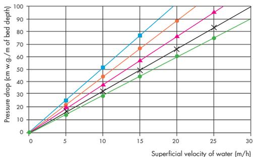
BED EXPANSION AND PRESSURE LOSS CURVES ARE PROVIDED FOR THE MOST COMMONLY USED PARTICLE SIZES. CHARTS ARE AVAILABLE FOR ALL PARTICLE SIZES ON REQUEST.
